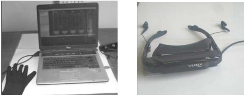
Figure 3. Components of a low – cost VR system: head-mounted display and DG5-Vhand glove
