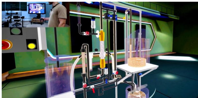
Figure 3. VR-based ultrafiltration scenario depicting membrane separation, valve configuration, and processflow visualization
