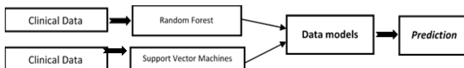
Figure 4. Scheme for late merging of results (Late Fusion from Scores)
